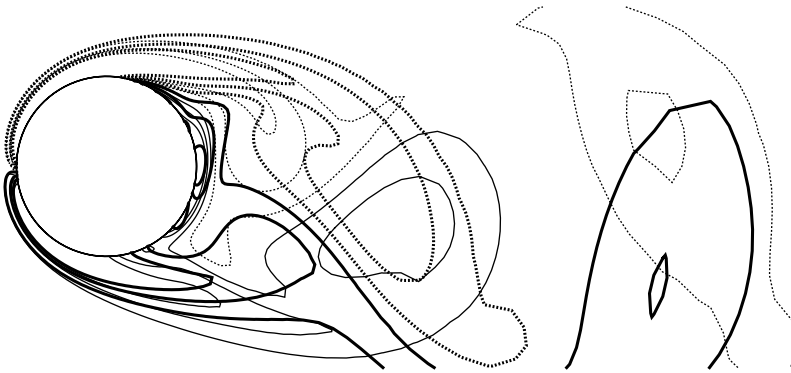
Figure 16. Superposition of the contours of constant vorticity at values of frequency ratio f_e/f_o = 1.00 (thick lines) and 1.12 (thin lines) for Re=185 and A_e/D=0.2 (—: positive values; ---: negative values). The location of the cylinder is at its extreme upper position.
